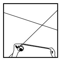
To determine the placement of the panel use a marker, a measuring tape and a ruler to mark the needed 4 points per panel on the ceiling. Placement aprox. 15cm from the vertices of the panel.
